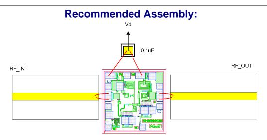
Figure 4 Assembly for single drain-bias operation
