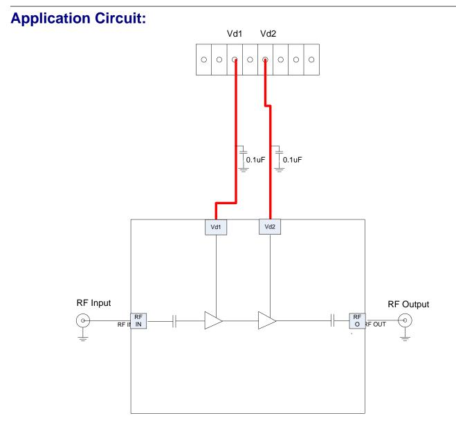
Figure 3 Application for single drain-bias operation
